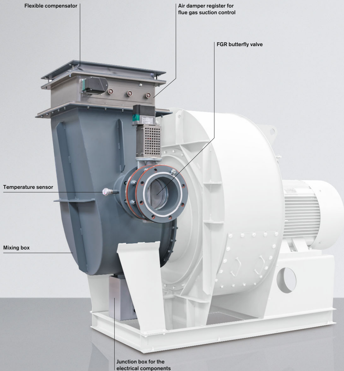
Mixing box for flue gas recirculation at the combustion air fan
