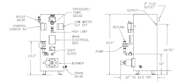
Note: Dimensions subject to change without notice. For ATM boiler, flue is 9" out the top, 6" if oil burner.
