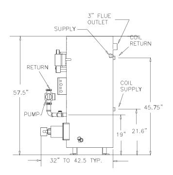
Note: Dimensions subject to change without notice. For ATM boiler, flue is 9" out the top, 6" if oil burner.
