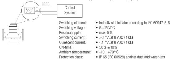
Connections: • Pulser supplied with special plug. Required cable min.
