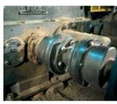
Close tolerances and registered fits allow Falk Freedom Disc Couplings to provide continuous high-speed service with virtually no maintenance.
