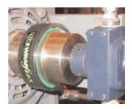
Wrapflex is a low cost, low maintenance, non-lubricated elastomer coupling from Falk. Quick, easy installation and replacement sets new standards for reduced downtime. Because motors don't need to be moved, our "replace- in- place" elements even eliminate the need for time consuming realignment. Falk Wrapflex Elastomer Couplings are backed by a 3- year warranty. Wrapflex is a great low cost, general purpose pump coupling!
